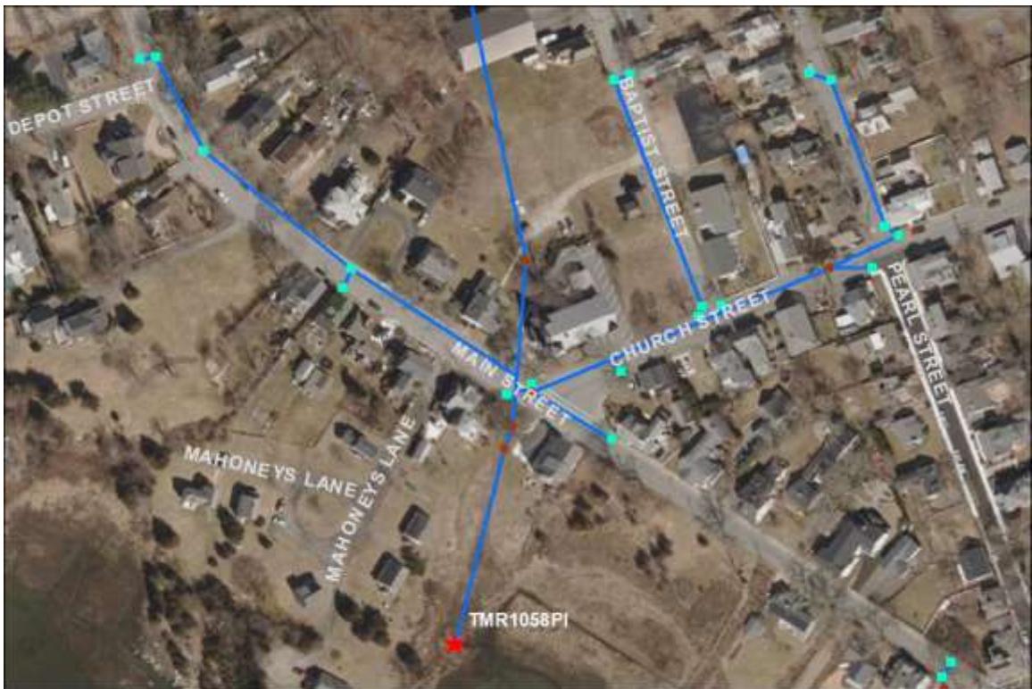
TMR1058PI – Main Street: no issues found; this is an extensive network and cumulates into a covered culvert with several pipes entering that cross Main Street; catchbasins on Church and Baptist Streets require cleaning.
